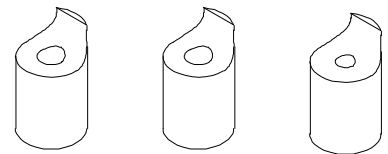
1.5 ml Microfuge Tube Holder, 8 mm Test Tube Holder, and 12 mm Test Tube Holder
